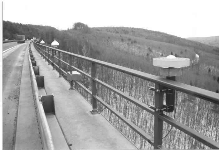
Fig. 2.7: Antennas installed on the southern railing in the middle of span 6
