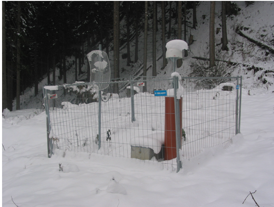
Fig. 5: GPS point 'Plateau' with tiltmeter and WLAN antenna.
