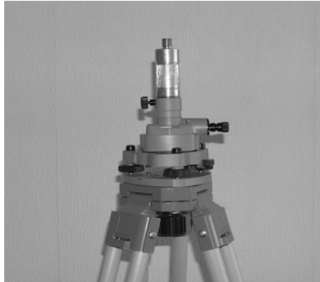
Figure 3: Prism and antenna adapter with optical plumb line
