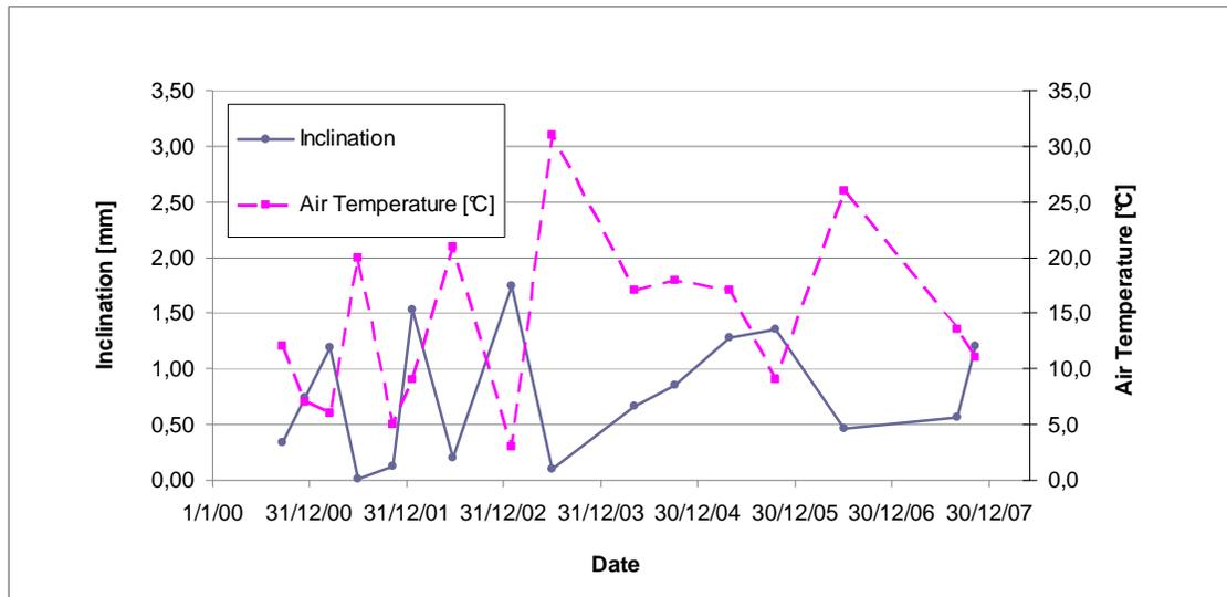
Figure 4 - Tilt of the pillar between measuring points 41 – 43 due to the outer air temperature
