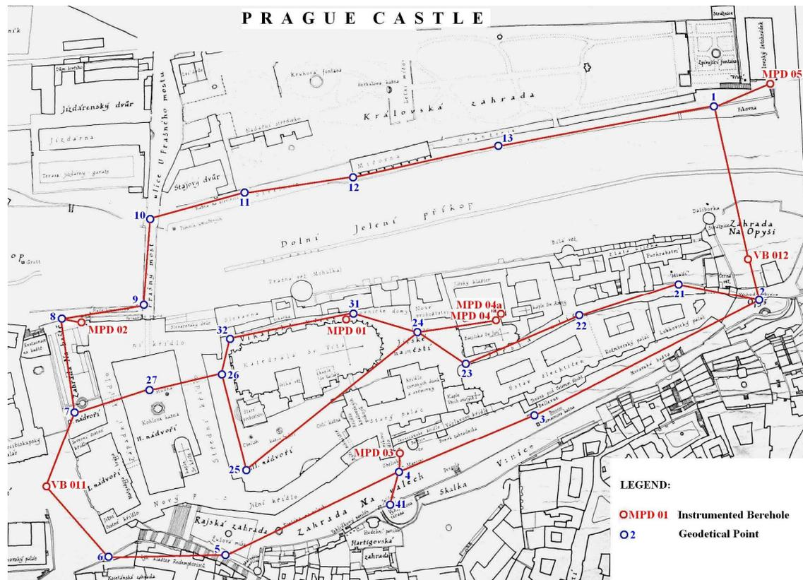
Figure 1 - Site plan of instrumented area of the Prague Castle
