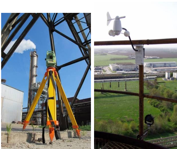
Figure 3. Total station (left) and prism with meteorological station on the top of the tower (right)
