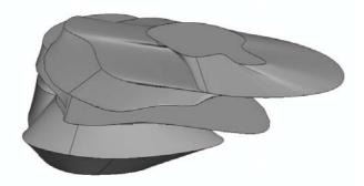
Fig. 1. Post-exploitation chambers measured with an echo-sonar
