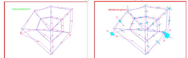
Fig. 6. Dislocation vectors and coordinates of the tensors of main strains
