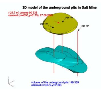
Fig. 2. 3D model of chambers and the subsidence on the surface
