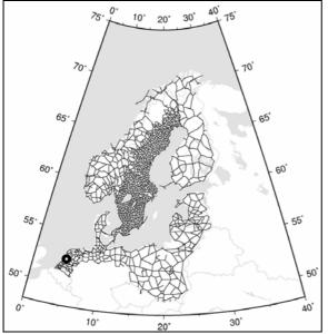
**Figure 4-1:** The Baltic Leveling Ring network. The zero point of it, NAP, is marked as a black ring on the map. (Mäkinen et al, 2005)
