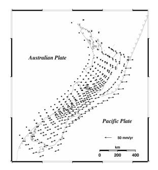
Fig 5: GNS deformation model showing horizontal velocities (Beavan 1998).
