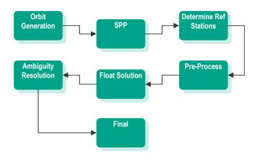
Fig 3: High level processing logic for PositioNZ-PP
