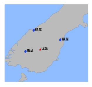
Fig 4: Example selection of three CORS within PositioNZ-PP
