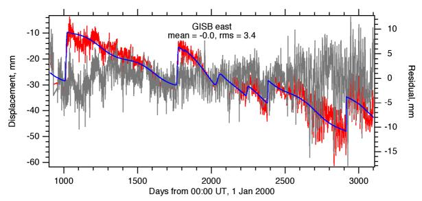
Fig 6: Plot showing the coordinate time series output (red), the models parameters (blue) and the residuals (grey) for the easting component of the PositioNZ GISB station. (Beavan 2008).
