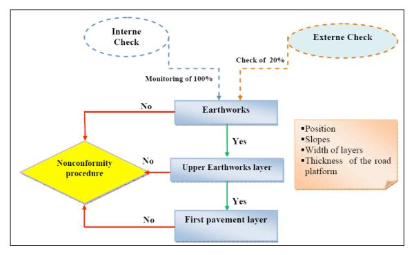
Figure 3. Earthworks monitoring and check process.
