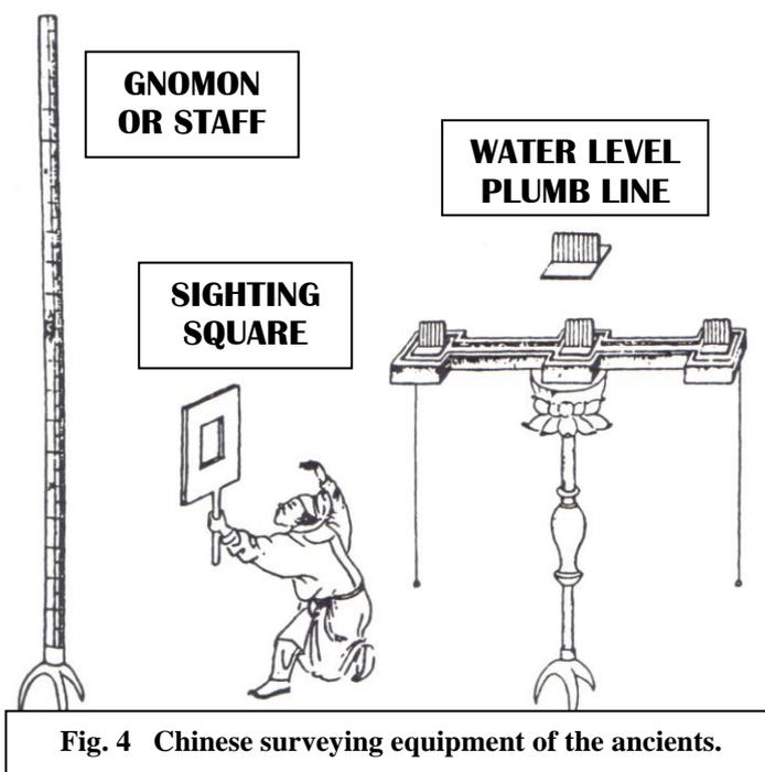
Fig. 4 Chinese surveying equipment of the ancients.
