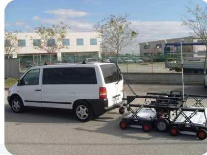
Stream EM System: complete configuration with 3 array of antennas
