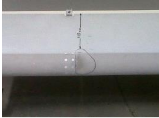
FIGURE 4. DENT ON A320 LEADING EDGE
