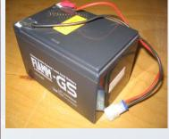
Power supply unit:2 batteries 12VDC 12Ah
