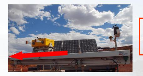
Using 2 m rail IBIS-L system obtains 4.38mrad (=0.25deg) angle resolution
