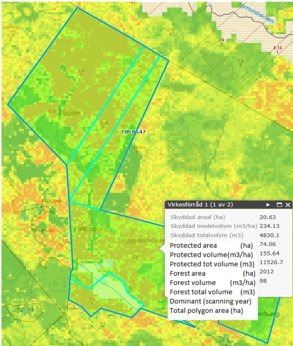
Fig. 13. Example of the result of a calculation of the standing volume. Here you can find the area and volume of protected forest and of unprotected forest and the year that is dominant in the laser scanning data (if the data originates from different years).
