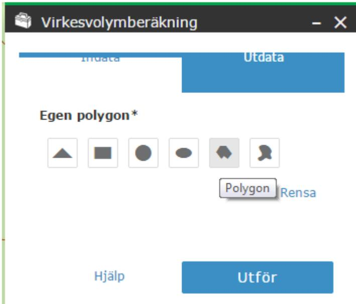
Fig. 15. Example of calculation of standing volume. Choose figure under "*Egen-polygon* - Custom Polygon" to "draw" the desired area to perform timber volume calculation on. The best option is Polygon.
