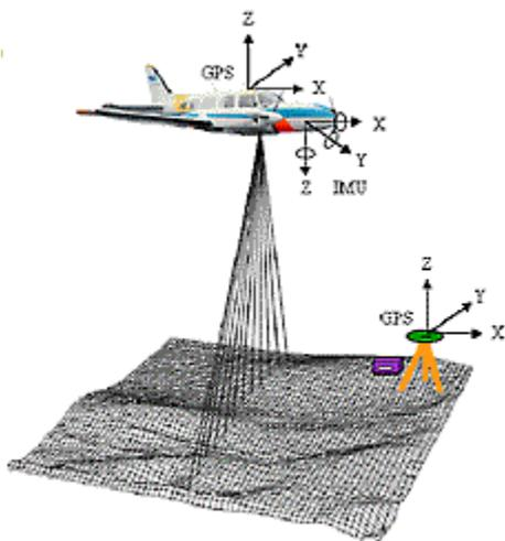
Fig. 1. Laser scanning from an airplane
