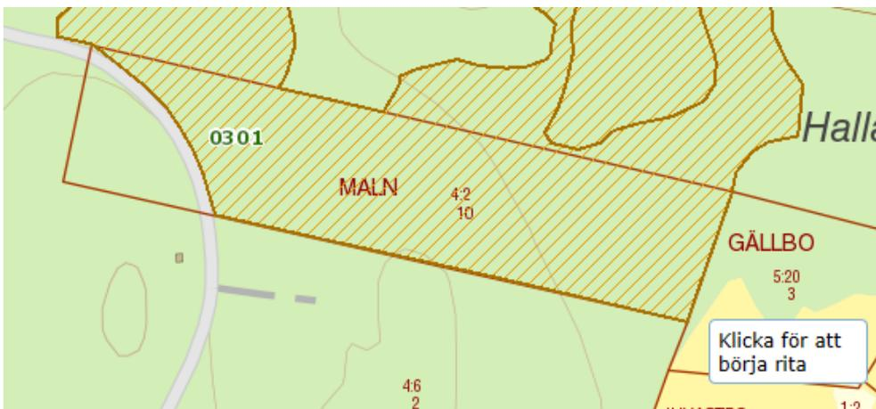
Fig. 16. Example of drawing borders. Start drawing the and with the click of the left mouse button, then proceed with the next boundary point etc. and finish the final figure with a double click. Then press button "*Utför*" to start the calculation.
