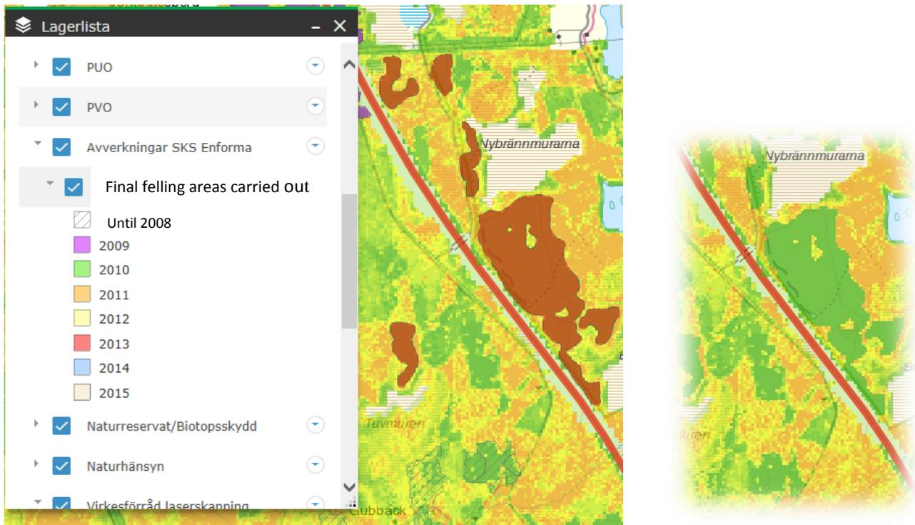
Fig. 6. Layer of recent final felling. If final felling is performed after laser scanning the volume is reduced to zero in the layer volume.
