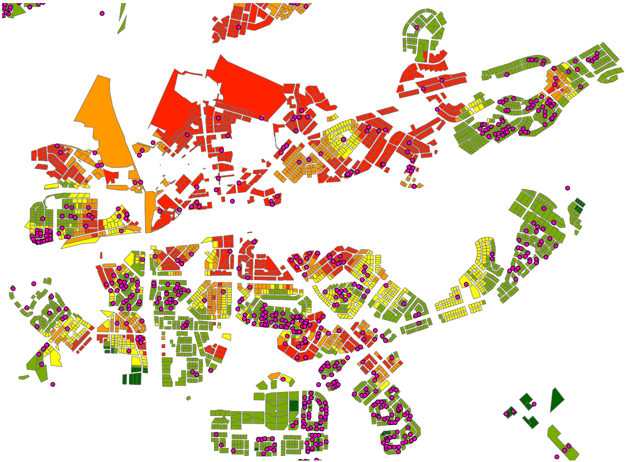
Figure 10. Based on three nearest neighbors a spatial moving average of land values is generated automatically.
