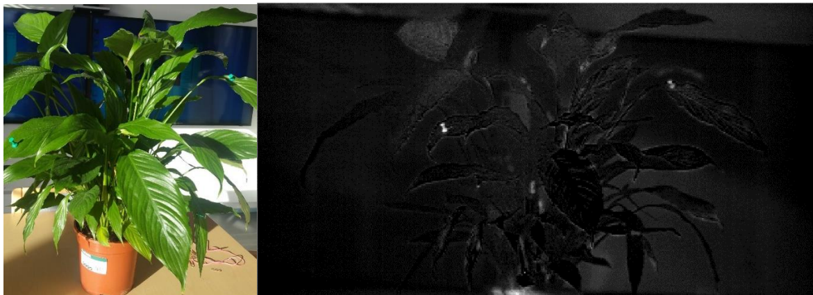
Figure 4. A photo and image of anomalous objects produced with unsupervised PCA filtering. To bring out the anomalous objects, a PCA transformation was done to the image, four most dominant spectral components were removed, and the PCA image was reverse-transformed back to normal hyperspectral spectral data cube. In the resulting data cube, the manmade anomalous objects (plastic pins and rubbers) are clearly showing up as they stand out spectrally from the majority of the scene. a). Plant with green pins; b) Plant with plastic buckets; c) PCA without any component removal; d) Investigate 12 top most dominant component contributions. The fifth component clearly shows the green pins; e) The seventh component shows the rubbers.
