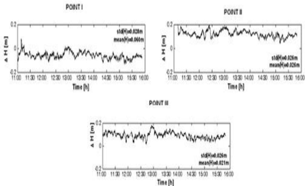
**Figure 6** Time series of epoch-to-epoch North, East and Height components in 3 May 2012
