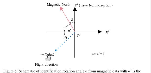
angle computed from calibrated magnetic data and  $\delta$  is magnetic declination angle
