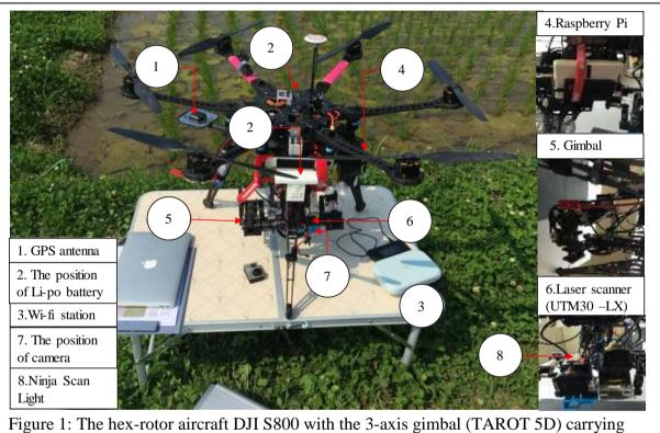
Figure 1: The hex-rotor aircraft DJI S800 with the 3-axis gimbal (TAROT 5D) carrying the Hokuyo UTM30LX laser scanner, an ultra-small motion logger (Ninja Scan Light), GPS receiver and a single-board PC (Raspberry Pi)
