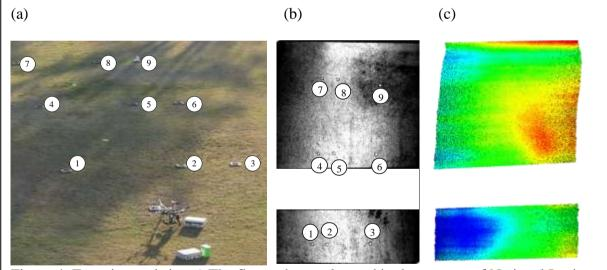
Figure 4: Experimental site. a) The flat study area located in the campus of National Institute of Technology, Kumamoto College, Kumamoto prefecture in Japan. There are 9 markers arranged on the ground surface for validating the accuracy of 3D point cloud generation, b) The intensity images and c) ellipsoid height of scanning points computed from observation data on Dec. 19<sup>th</sup>,2014 respectively, color coded (red= high, green= low).
