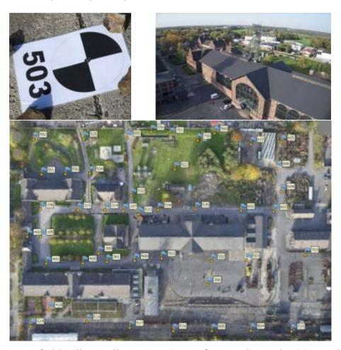
Fig. 2: UAV test field Zollern colliery. Top: Target for signalizing the GCPs and view of the area. Bottom: Point cloud with signalized GCPs (UAV flight from October 2017)
