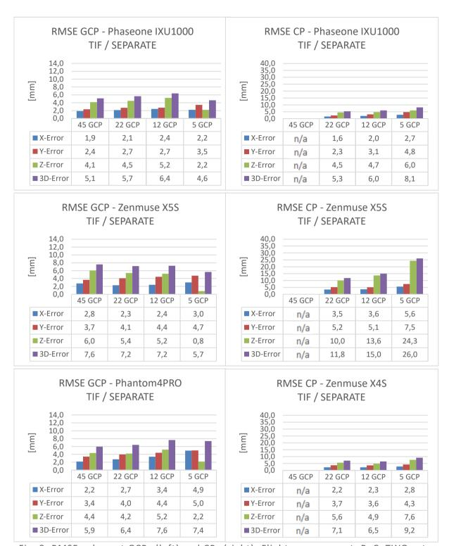
Fig. 8: RMSE values at GCPs (left) and CPs (right). Flight arrangement: R+C. TWO sets of interior orientation parameters (SEPARATE). Calculation: Agisoft PhotoScan. Note scaling.
