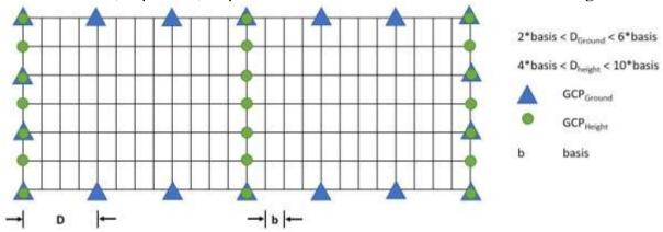
Fig. 6: Schematic arrangement of GCPs during (analogue) image flight (Kraus 1994)
