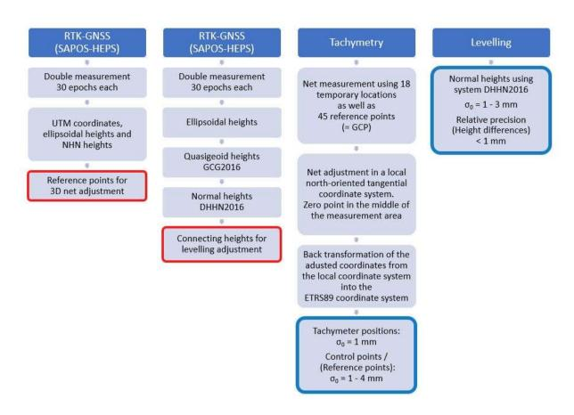
Fig. 3: Workflow of geodetic measurements and data processing (GCG2016 - German Combined QuasiGeoid, the height reference for the transition between geometric heights in ETRS89/DREF91 and physical heights in DHHN2016, the German height reference system).
