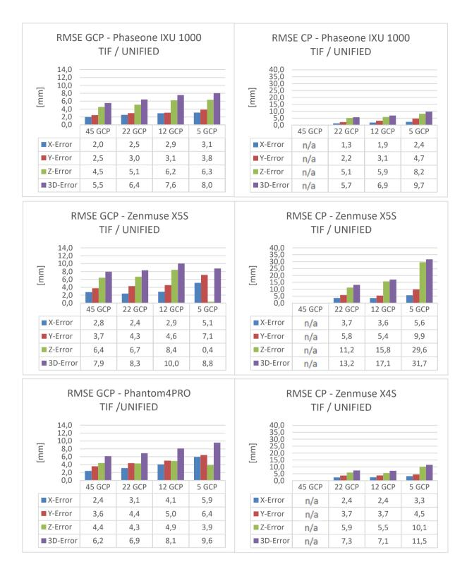
Fig. 7: RMSE values at GCPs (left) and CPs (right). Flight arrangement: RC. ONE set of interior orientation parameters (UNIFIED). Calculation: Agisoft PhotoScan. Note scaling.
