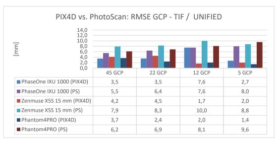
Fig. 10: Comparison of the 3D RMSE values at GCPs (top) and CPs (bottom) as results of
