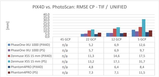
the bundle block adjustments with PIX4Dmapper and Agisoft PhotoScan. Note scaling.
