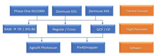
Fig. 5: Parameters influencing the geometric quality of the image blocks
