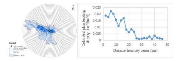
Figure 4 Schematic diagram of downtown buffer analysis
