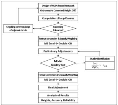
Figure 7. A procedure of UCPs-based levelling network adjustments. **3.2 Examination of Loop Closures**
