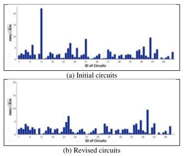
Figure 9. Standardised misclosures of the circuit loop closures.
