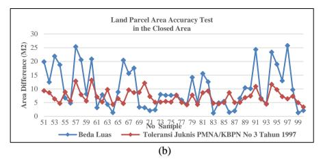
Figure. 2. The area accuracy test results in the area of (a) opened and (b) closed
