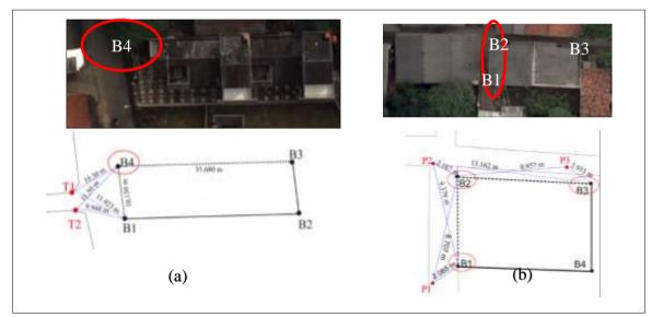
Figure. 3. (a) Determination of land parcel boundary B4 with methode of "pemotongan kemuka" (b) Determination of land parcel boundary B1, B2, and B3 with combination method of GNSS and Terrestris
