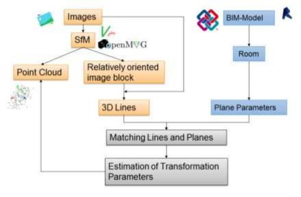
Fig. 6: General workflow of the proposed concept
