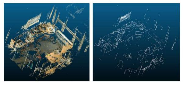
Fig. 5: Generated dense point cloud of a room (left) and extracted 3D line structures (right)
