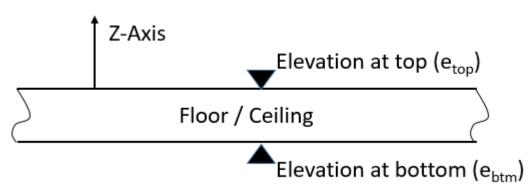
Fig. 2: Sideview of a Floor or Ceiling element. Planes from the object (floor/ceiling) must be carefully selected by any algorithm
