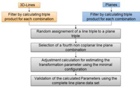
Fig. 7:Basic workflow for the transformation parameter estimation
