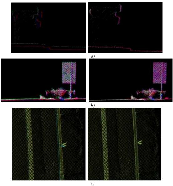
*Figure 1. Point cloud matching results – a) Curb detail; b) Road profile and traffic sign; c) Guardrail fence and white line on the road (top view)*
