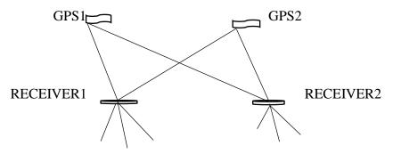
Figure 2: Double differencing; Source: Eissfeller et al. (2011)
