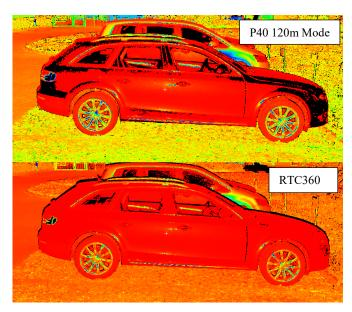
Figure 5: Comparison of the same scan of a black car performed with ScanStation P40 and RTC360.
