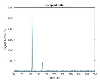
Figure 4: Emitted EDM pulses on RTC360.
