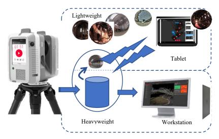
Figure 9: Data transmission and synchronisation between the three components of the RTC360 solution.
