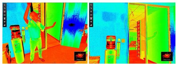
Figure 13a and 13b: Effect of the moving object filter in Cyclone REGISTER 360.
