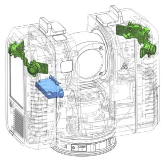
Figure 6: Hardware components of the Visual Inertial System.
