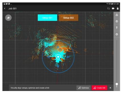
Figure 10: Visual alignment in Cyclone FIELD 360.
