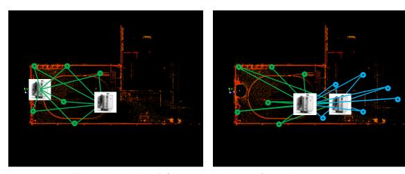
Figures 8a and 8b: 3D features resection and forward intersection.
