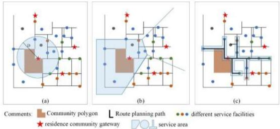
Figure 4. Schematic diagram of the methods used to calculate the accessible public service facilities
