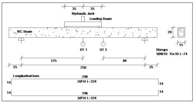
Figure 1: Test set-up
