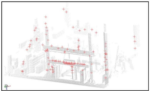
Figure 2: Measurement points for the Laser Tracker and the VMS AICON DPA
