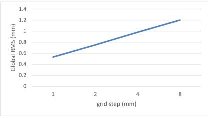
Figure 12: Global RMS vs TLS grid step in mm
