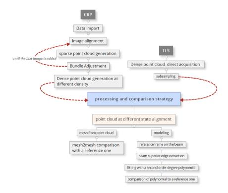
Figure 7: Processing strategy for CRP and TLS
