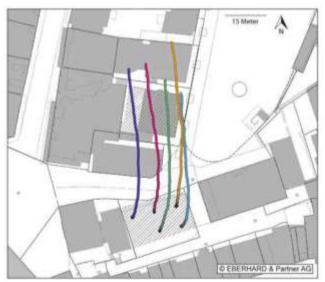
Figure 2: Probe course in the depth shows drift over neighbouring plots of land
