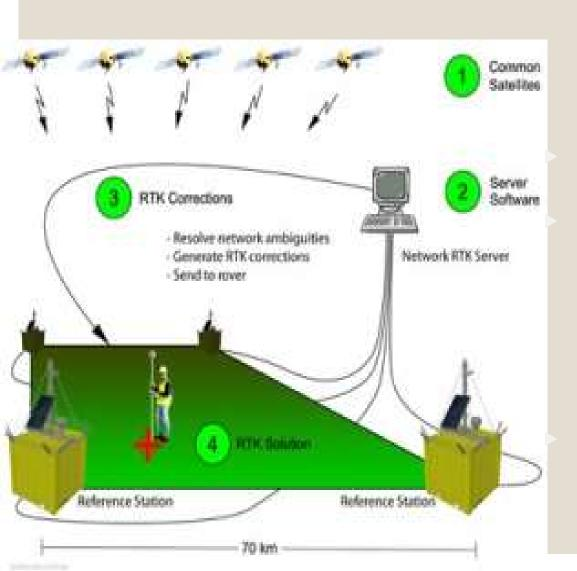
CORS GNSS Network is used for providing fit-for-purpose positioning.
