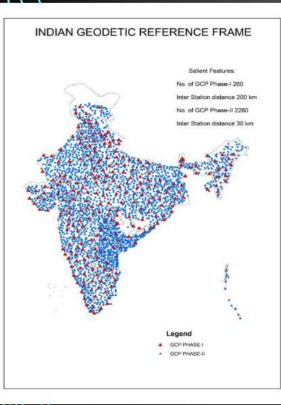
Indian geodetic reference frame (IGRF) was established through a "passive" network about 260 well spread Ground Control Points (GCPs) at a spacing of 250-300 km apart across the country during the period from This network was observed and adjusted in combination with few IGS stations surrounding the Indian territory. The current Indian horizontal reference frame is linked to the International Terrestrial Reference Frame (ITRF) The network was further densified with 2260
