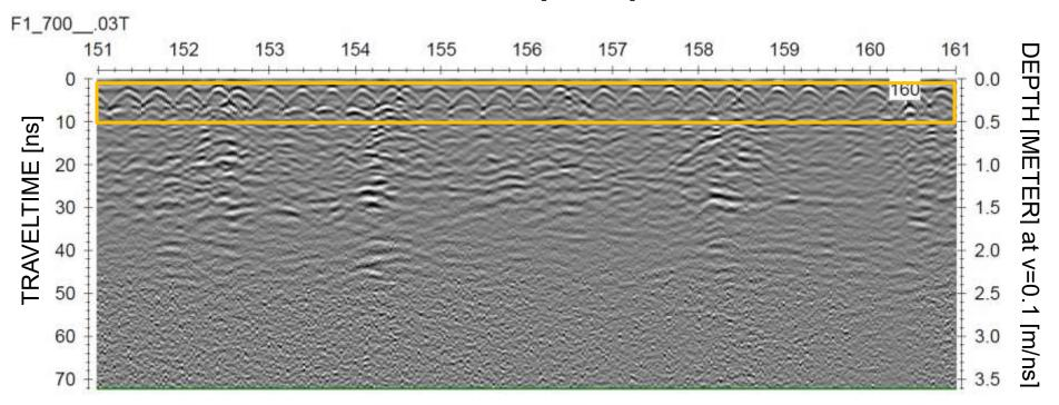
Reinforcing bar's are located at the top of each hyperbola
