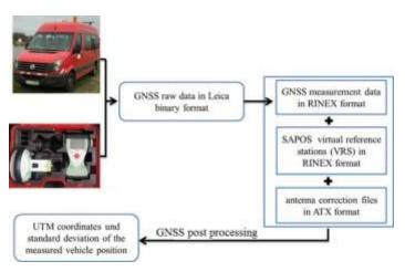
Generation of reference Trajectories based on kinematic GNSS measurements
