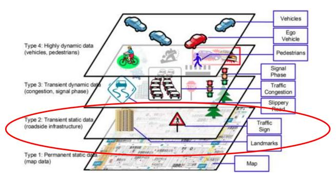
The layered architecture of the LDM (Source: Schimada et al., 2015, "Implementation and Evaluation of Local Dynamic Map in Safety Driving Systems". Journal of Transportation Technologies, 2015, 5, 102-112)
