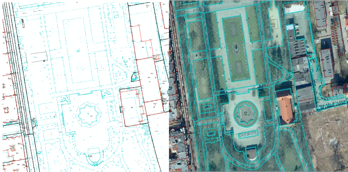
Fig. 2. Updating the BDOT500 database using photogrammetric data.
