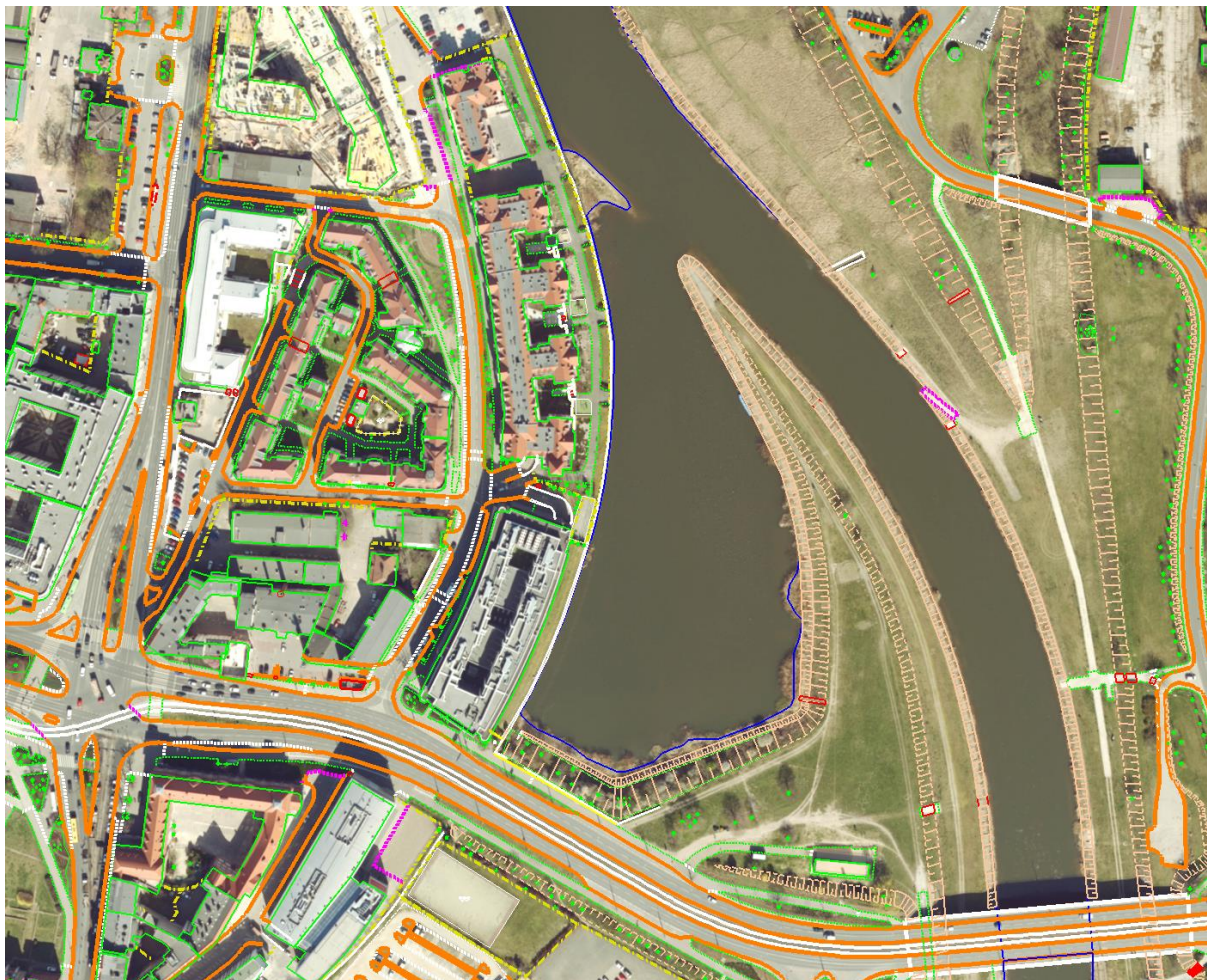
Fig. 1. Vector data acquired by stereodigitization of aerial photographs.
