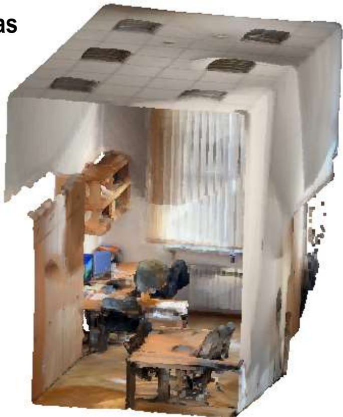
Colored point cloud view of the section of an office room scanned by the iPhone 13 Pro
