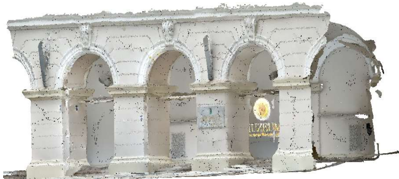
Colored point cloud of a fragment of the main hall of Warsaw University of Technology scanned by the iPhone 13 Pro
