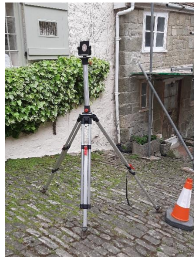
Figures 4 & 5. Typical scanning targets used for survey control. (Author's Image, 2022)
