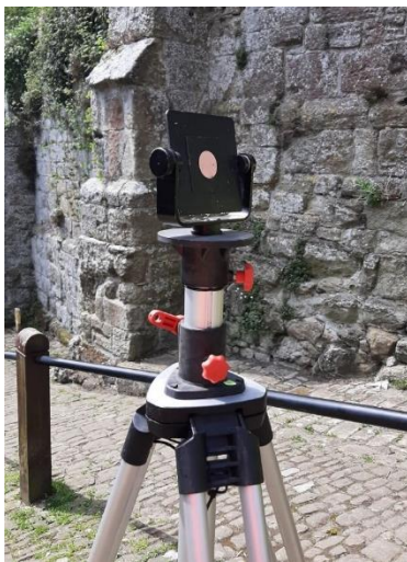
Figures 4 & 5. Typical scanning targets used for survey control. (Author's Image, 2022)
