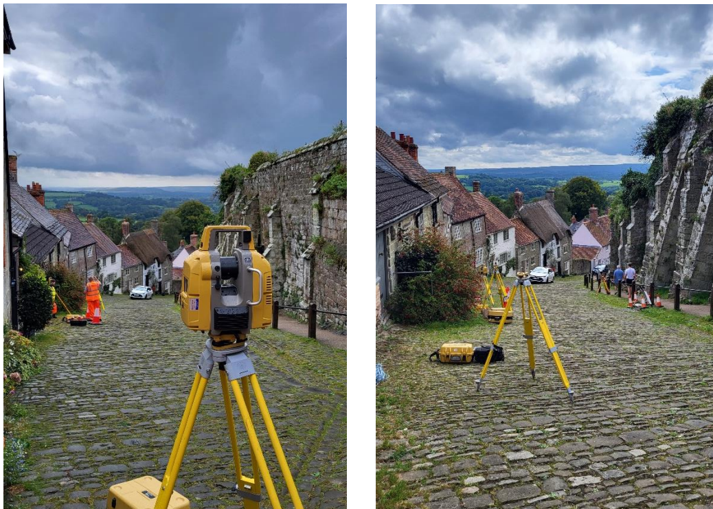
Figure 5 & 6. The GLS-2000 scanner and the station setups on site – the retaining wall can be seen to the right. (Author's Image, 2023)
