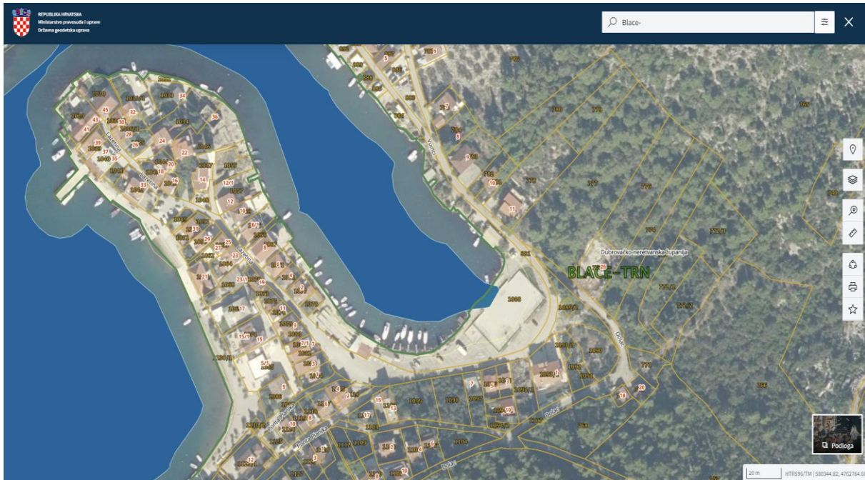
Figure 3. Cadastral map of real property cadastre, scale 1:1000 - cadastral municipality Blace-Trn (source: https://oss.uredjenazemlja.hr/#/ )
