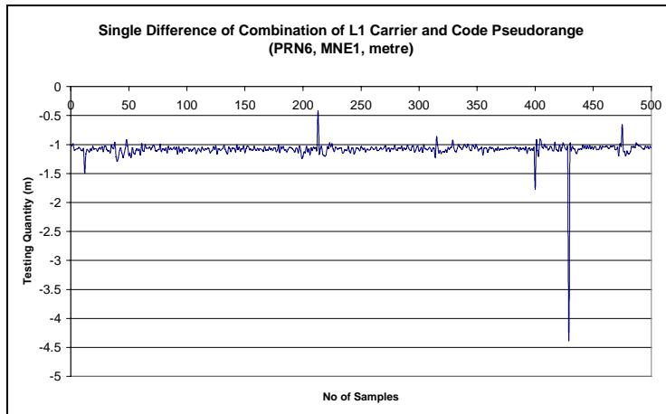
Figure 11. Single difference of L1 carrier and pseudorange
