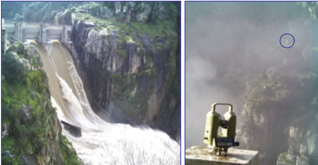
Figure 4 – Water vapour, resulting from the discharge of the reservoir, affecting the optical path between two station points.
