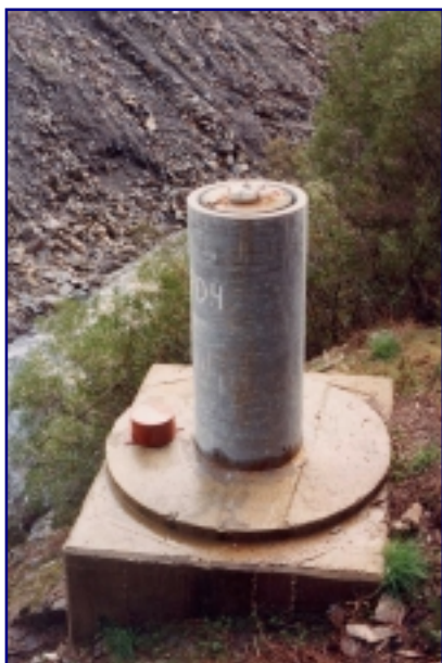
Figure 2 – Concrete Pillar with foundation.
