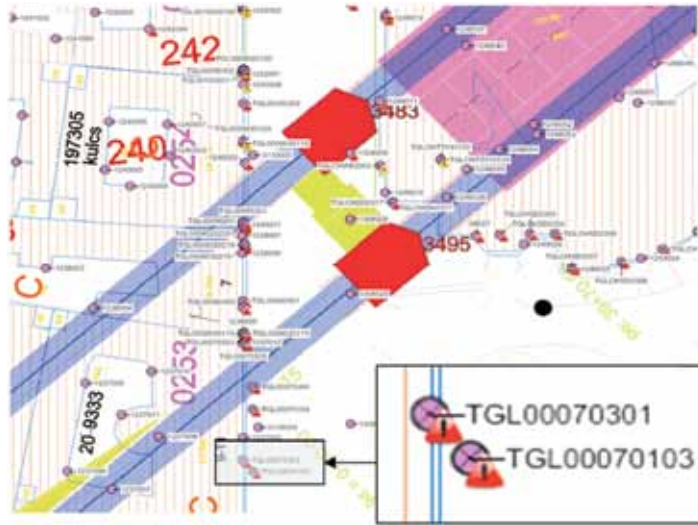
Figure 4: Kronos user interface showing a live-map situation of Budapest city with monitoring points in alarm status while two tunnel boring machines are excavating underground.
