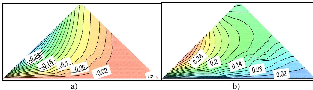
Figure 2 - Predicted displacements [m] after filling the reservoir a) vertical displacements
