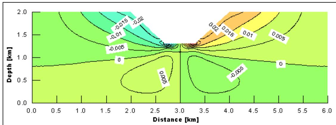
Fig. 4 - Horizontal displacement [m].
