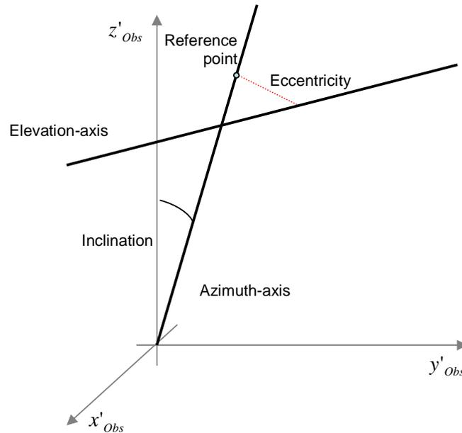
Figure 1 - Restrictions (eccentricity and inclination), for clearness shown in the coordinate system  $x'_{Obs}$ ,  $y'_{Obs}$ ,  $z'_{Obs}$ , which emanates from the observation system  $x_{Obs}$ ,  $y_{Obs}$ ,  $z_{Obs}$  by translation
