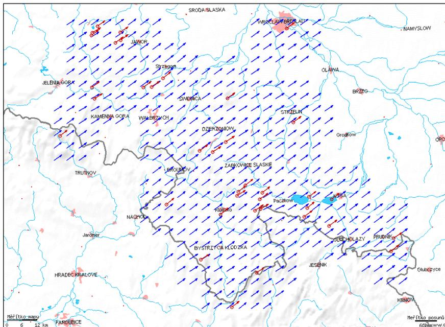
Figure 8 - GEOSUD network, displacement field in ITRF 2000
