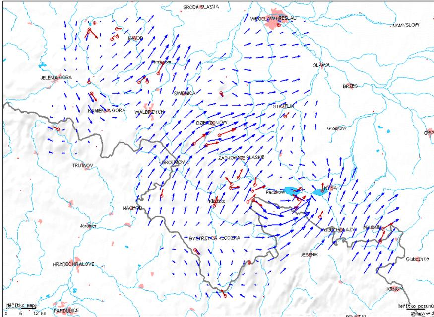
Figure 9 - GEOSUD network, displacement field in “local” system
