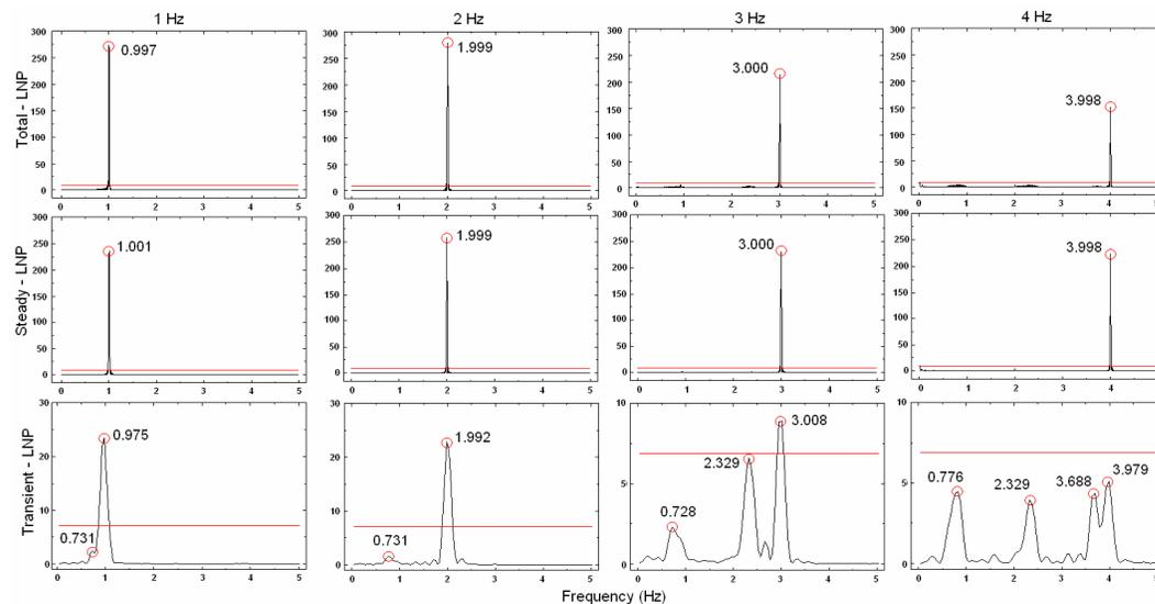
Figure 3 - Spectra of GPS time series of representative experiments for constant excitation of 1, 2, 3 and 4 Hz. The first row corresponds to the spectra of the whole time series, the second
