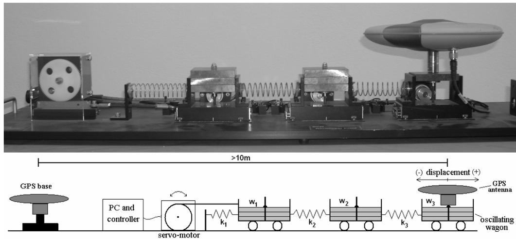
Figure 1 - A photo of a part of the oscillation device and a sketch describing the instrumentation used in our three-degree of freedom oscillation experiments. The GPS rover antenna is settled on the third wagon. All the wagons ( $w_1$ ,  $w_2$ ,  $w_3$ ) are connected with springs ( $k_1$ ,  $k_2$ ,  $k_3$ ).
