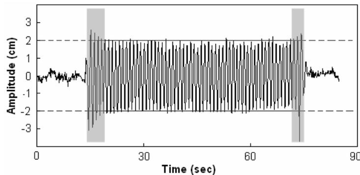
Figure 2 - A representative GPS time series of the oscillation displacements indicating with the two gray zones the initial and the final parts of the time series and the middle part corresponding to the steady oscillation
