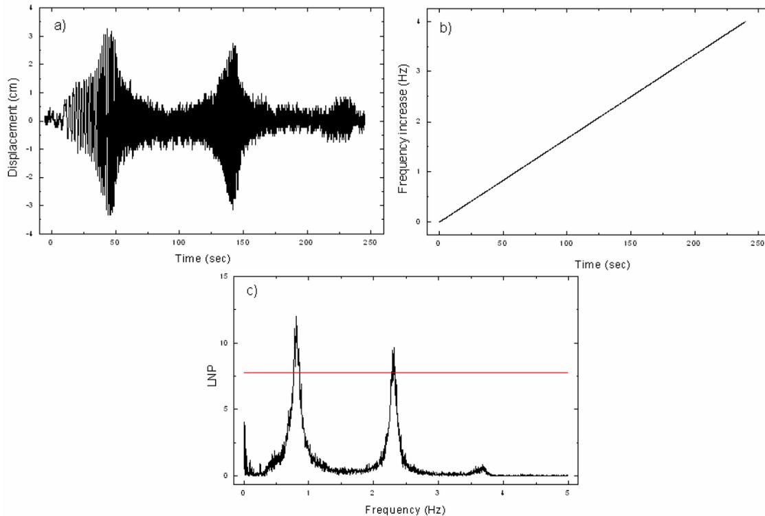
Figure 4 - Results of an experiment with three degrees of oscillation and frequency increasing linearly from 0.05 Hz to 4 Hz in 4 minutes. (a) Displacement, (b) real oscillation frequency and (c) computed frequencies using the Normperiod Code (LNP spectrogram). Three displacement peaks are observed in the displacement diagram, indicative of resonance. The two lower modal frequencies are clearly shown in the LNP spectrogram, while the third one is shown as a minor peak.
