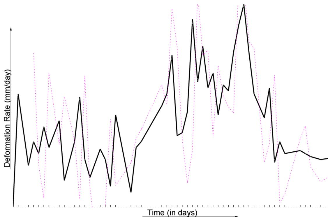
Figure 1 - Deformation rate of bench in Megalopolis lignite mine
