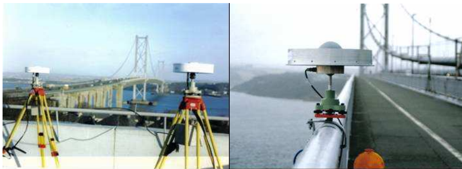
Figure 11 - Two GPS reference receivers located adjacent to the Forth road bridge (left). A GPS choke ring antenna attached to the bridge (right).
