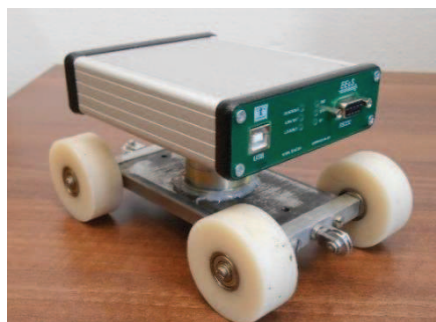
Figure 5 IMU EEaS placed on cart
