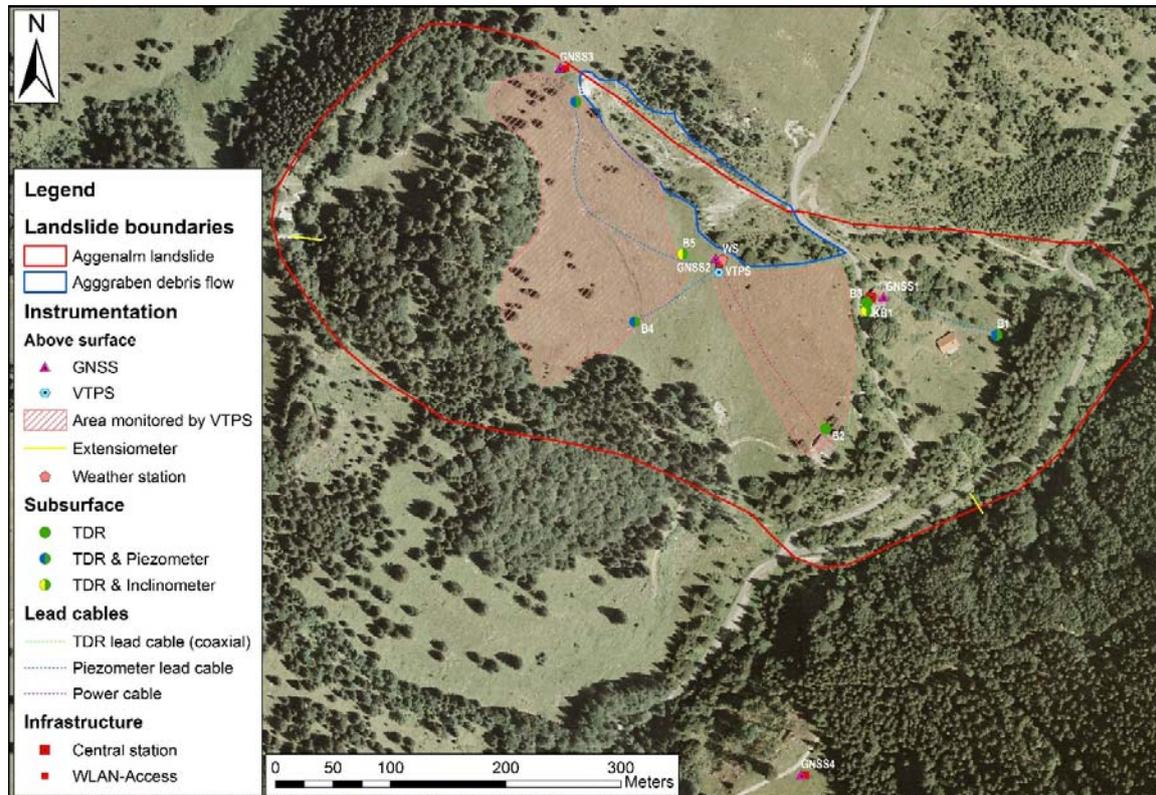
**Fig. 1** Orthophoto of the Aggenalm Landslide (red boundary) and the 1997 debris flow (blue boundary) superimposed by the elements installed and used during the alpEWAS project (Singer et al. 2009).
