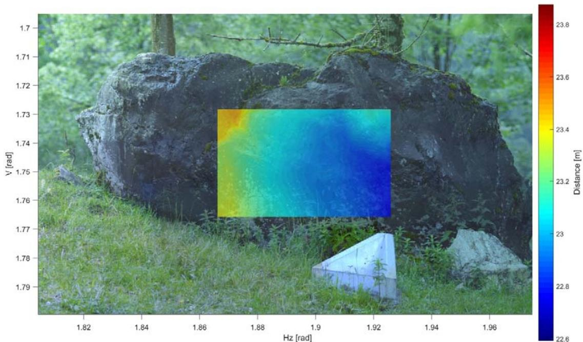
**Fig. 3** Spherical panorama composed of 9x7 telescope camera images using a Leica MS50. Column pixel coordinates correspond to horizontal angles, rows to vertical angles of the theodolite. A part of the scene is superimposed (faded) by the color coded D-channel, which represents the distance from the station to the respective pixels.
