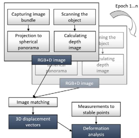
**Fig. 4** Sequence diagram of the new geo-monitoring approach based on RGB+D images (Wagner 2016).
