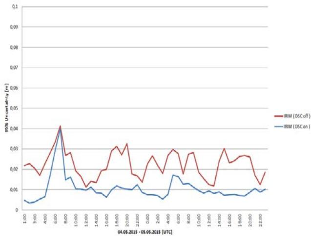
**Figure 5: Predicted ionospheric error for Network Processor, with DSC disabled and enabled**
