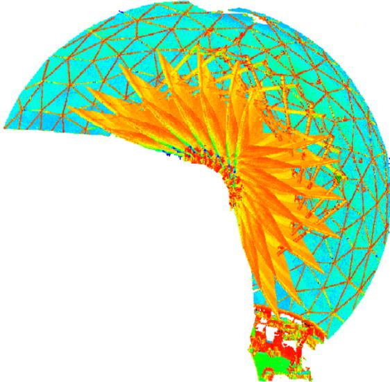
Figure 6. Transformed point clouds (all 7 elevations) into one stable reference coordinate system (Holst et al., 2019)
