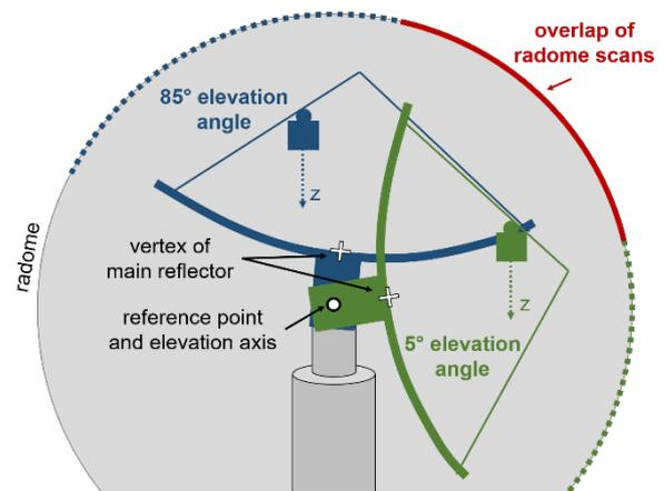
Figure 2. Measurement concept of scanning the OSO 20-m radio telescope; edited from Holst et al. (2019)
