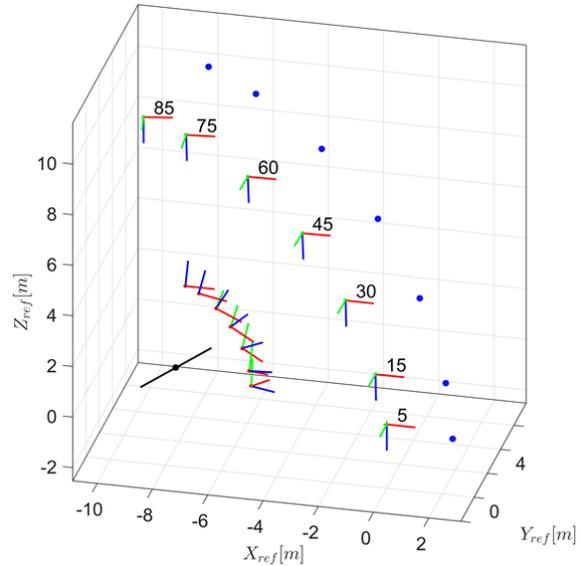
Figure 7. Estimated elevation axis (black line), reference point (black dot), vertices of the main reflector (tripods without labels of elevation angles), laser scanner stations (tripods with label of elevation angles) and focal points of main reflector (blue dots) (Holst et al., 2019; edited from Holst et al., 2019)
