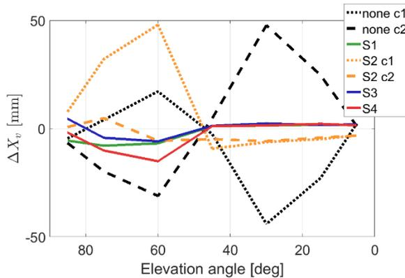
Figure 5. Relatively estimated translations in X-direction between laser scanner station and vertex of the main reflector.
