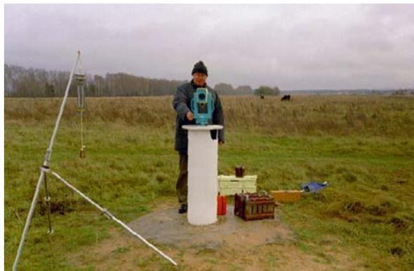
**Fig. 10.** Measuring a calibration baseline and test field in Lithuania.
