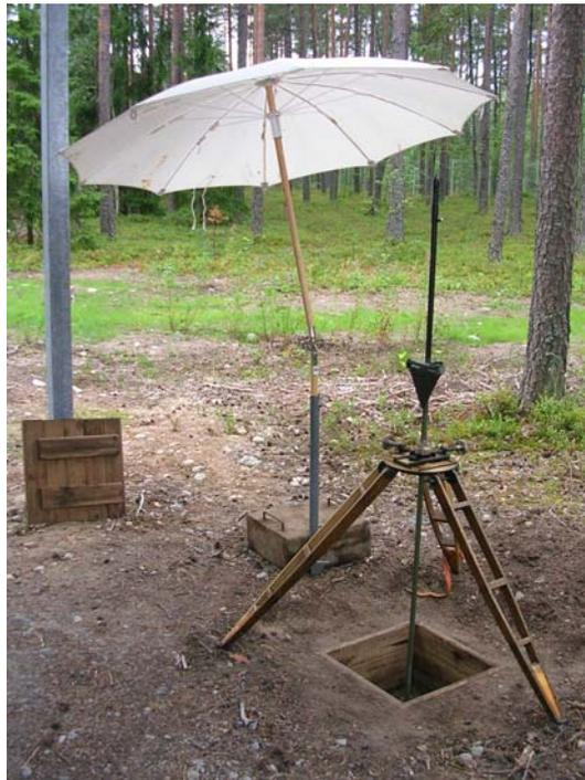
**Fig. 5.** Reaching for an underground marker at 0.01-mm-level by mechanical plumbing.
