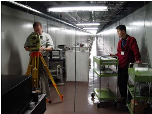
**Fig. 11.** Measurements at the NMIJ/AIST baseline in Tsukuba, Japan.
