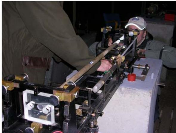
**Fig. 7.** Working with the Väisälä comparator.
